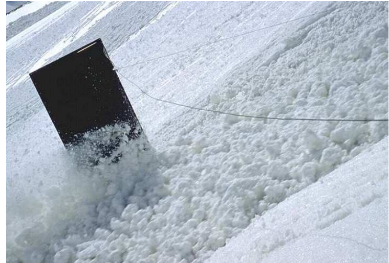
Dense flow avalanche impacting a deflecting structure
